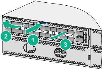
① Press the latch on the card to release the ejector lever.
