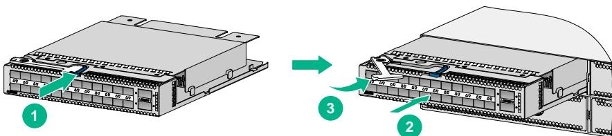
① Unpack the card. Press the latch on the card to release the ejector lever.
